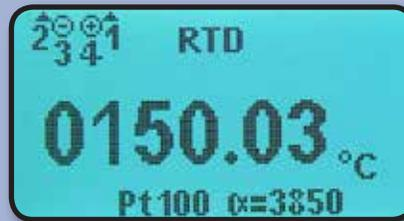
Here is an example where connections are made to a 4 wire sensor and the PIE 525B indicates that only Wires 1, 2 & 4 are connected. There may be a loose connection or a break in wire 3 somewhere between the sensor and the 525B.
